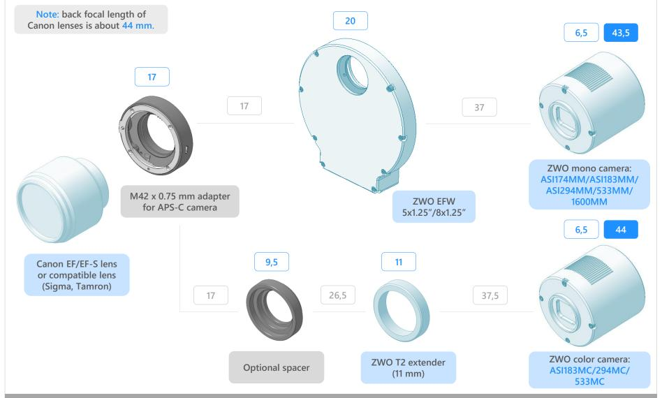
You only need the base adapter to use your camera with a filter wheel. An additional spacer is needed for cameras without a filter wheel (e.g. color cameras).
