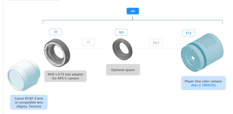
An additional spacer is needed for cameras without a filter wheel (e.g. color cameras).
