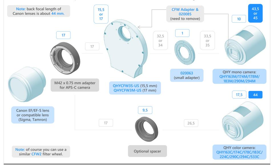
An additional spacer is needed for cameras without a filter wheel (e.g. color cameras).
